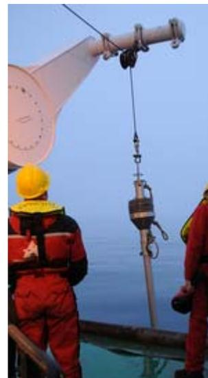
*deploying the gravity corer*
